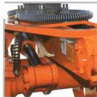
The hoses are carefully routed and protected with a spiral guard against damages.
