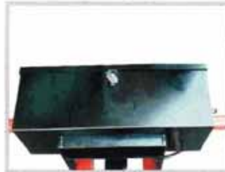
Hydraulic System: Contains Motor & Pump; Operates ram to fold up and cradle for loading and carrying.
