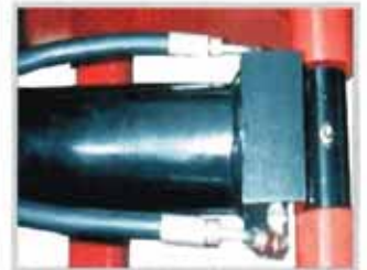
Pilot operated holding valve on cylinder, flow check valve on pump ensures load holding both ways!
